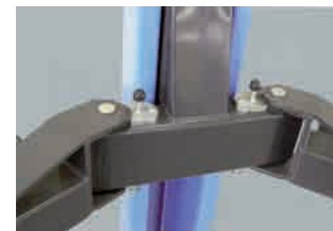
Self-lock/unlock arm system in lifting mode/reach the floor mode
